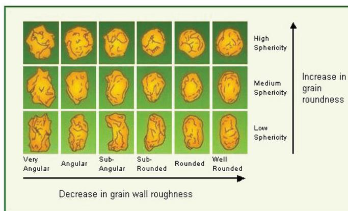
Grain shape refers to two attributes: surface texture or angularity and grain roundness or sphericity. Grain shape is determined by nature and is dependent on the weathering and erosion subjected
