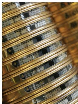
is then mechanically shaken through a stack of sieves. Various sieve mesh sizes are used depending on grain size distribution of the material being tested. If the material contained clay or organic material it would be washed and dried prior to sieve analysis testing otherwise the grains would stick together giving a false result.
